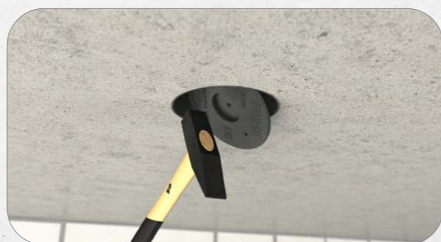
10. Simple opening of the Front Part with a hammer blow after concreting.
