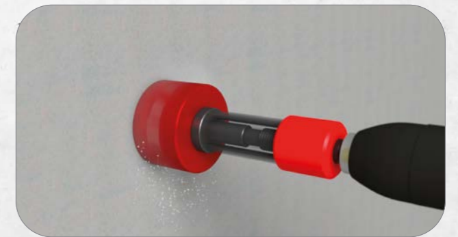
4. Place the box mill in the centering hole and mill out the hole.
