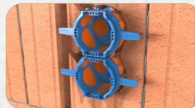
3. Securely connect the Thermo Boxes with a 71 mm combination spacing and insert them into the drilled hole. A flush finish is guaranteed thanks to the plaster stop.
