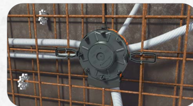
2. Open the membrane with a cutter knife. Combination entry of cables and (rigid) conduits from M9 - M40 without tools. The membrane technology guarantees absolute concrete-tight entries.
