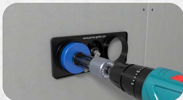
3. For multiple combinations, insert the Drilling Template (P102-74) into the first hole. Align it using the integrated spirit level and tighten the lever. By repositioning the Template, drill any number of additional holes at the standardized 71 mm spacing.
