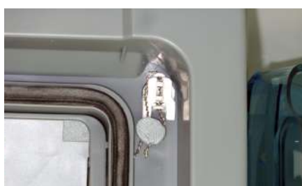
Sealing the screws on the front panel
